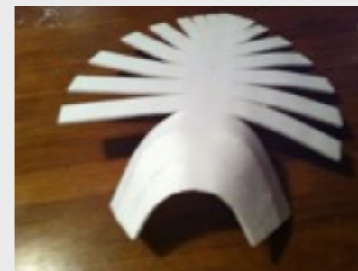
FIGURE 2.9 Four relief cuts closed
