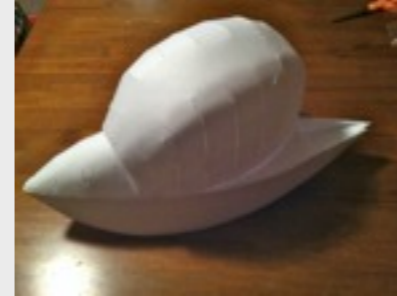
FIGURE 2.12 Glue cockpit right against nose cone
