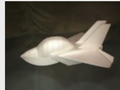
FIGURE 3.8 Forward fuse level with wing
