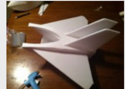
FIGURE 3.5 Fuse top and vert stabs in place
