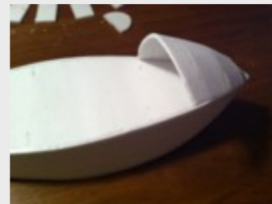
FIGURE 2.6 Nose being glued on
