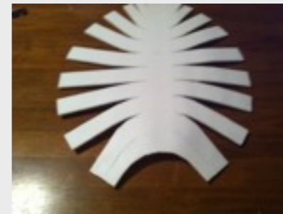
FIGURE 2.8 First two relief cuts closed
